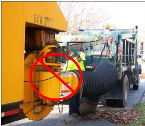
Visibility of the workers on foot is a critical component for a safe operation. In the picture on the left, the worker is between the leaf vacuum and the truck and out of the driver's sight.
